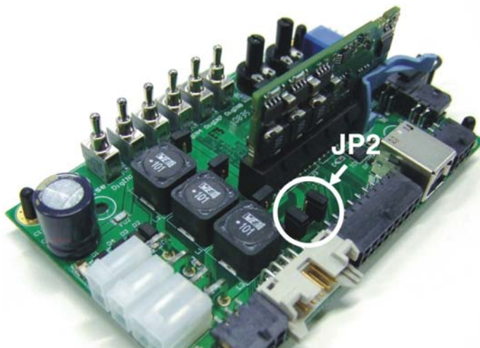
Figure 3-2 Jumpers JP2a/JP2b (Location and Factory Setting)
